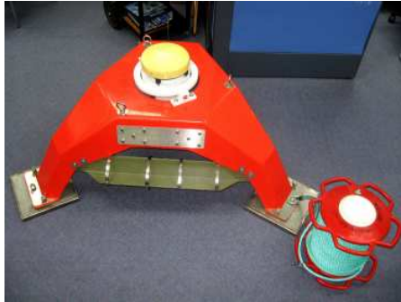
A Sea Spider frame with bracket ready for the RBR Tide Gauge. (picture courtesy of the RAN)
