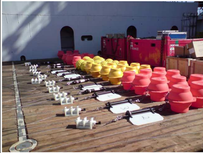
12 RBR CTD's ready to be deployed on a 1,200m mooring.
