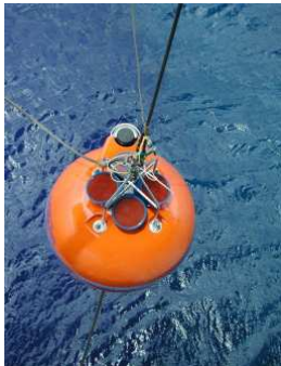
75 kHz ADCP being deployed from a rig (see page 2) -picture courtesy of RD Instruments.
