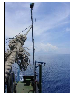
Cnav DGPS installed next to over-the-side ADCP mount
