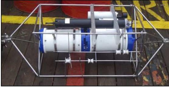
The rig is due to arrive at location later this month but prior to this, the rigs anchors will be pre-laid. Due to the lack of quality data for this location, MSI have deployed the current profiler from a vessel moored to one of the anchor buoys to gather as much data prior to the rigs arrival.
