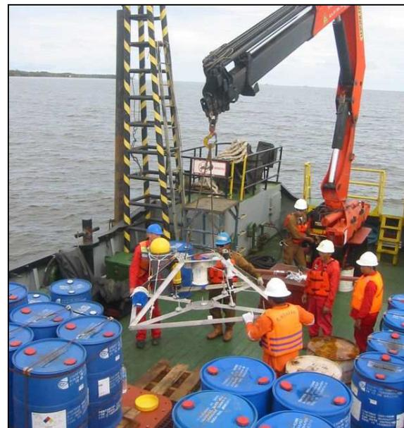
The second project is the provision of real-time current measurements to support a drilling campaign offshore North Lombok. MSI will install a TRDI 75kHz acoustic Doppler current profiler to measure multi layer currents in 600m of water whilst the rig is drilling a single well.
