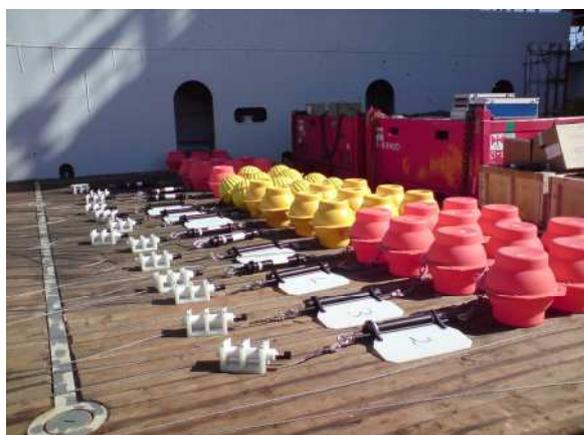
The mooring was deployed in August 2008 using the vessel MV Siem Louisa and serviced in November 2008 using the MV Ocean Prince, and comprises a TRDI 300kHz ADCP, 14 Nortek Aquadopp current meters and 15 RBR Ltd XR420 CTD loggers.
